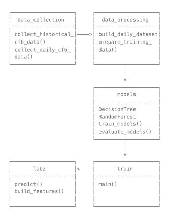
This UML diagram represents the flow of data and control in the weather prediction system. The modular design allows for clean separation of concerns, making the system easier to maintain and extend.
